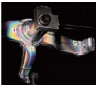
Figure 6 – Analysis of stress tendency in an automobile steering knuckle
