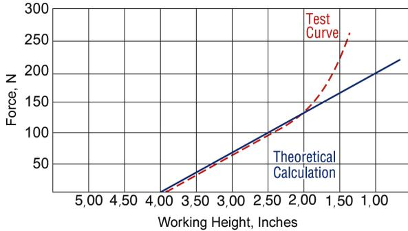
Figure 10 – Deflection characteristics, Theoretical and Measured
