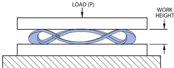
Figure 4 – Load Requirement
