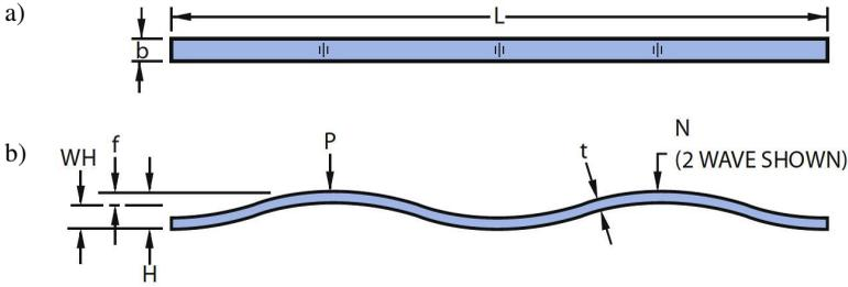
Figure 9 – Linear Expander: *a* – Plan; *b* – Side view
