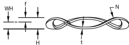
Figure 5 – Single Turn wave spring
