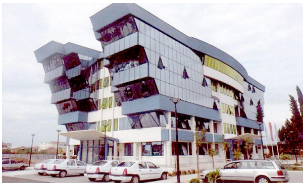
Figure 5 – Building with the 1,6 \text{ W/m}^2\text{K} thermal diffusion coefficient (Semi Structural Solar Facade Serial ALUMIL M3 alutherm [7])
